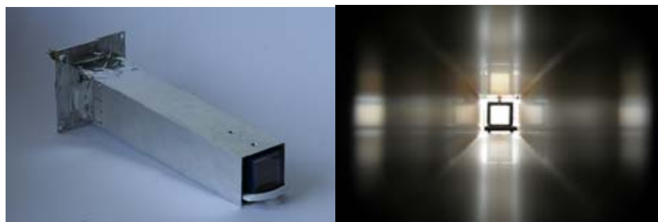
Fig. 4 (left) The Mini2 LE objective is focal length of 250 mm suitable for application in micro and picosatellites. and Fig. 5 (right) The inside view of the Mini1 LE module
