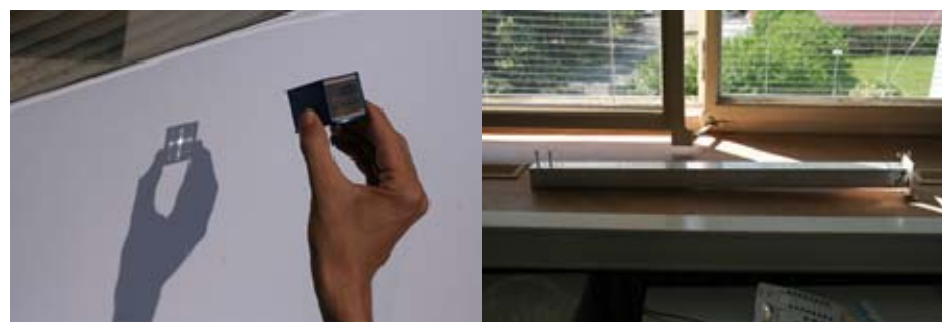
Fig. 6 (left) Imaging properties of the Mini2 LE system – imaging of the Sun in optical light and Fig. 7 (right) The Mini1 LE module with focal length of 900 mm.
