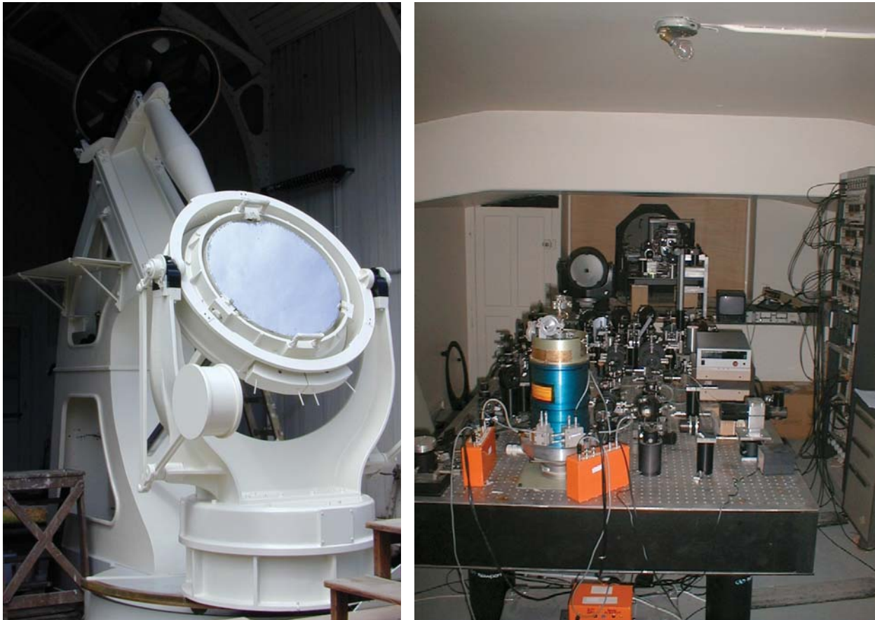
Figure 6 "Grand Sidérostât de Foucault" and the 3 telescopes breadboard demonstrator at Meudon Observatory.
