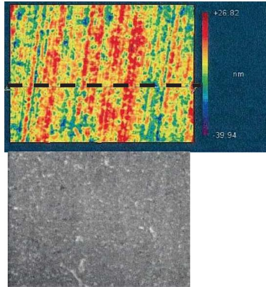
Fig. 8: Height Map (upper panel) and Intensity Map (lower panel). Surface Finished by #4000 Disk Grindstone.
