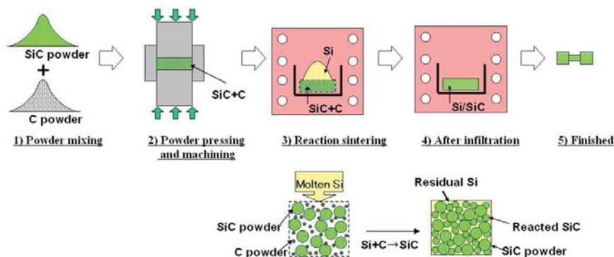
Fig.1 Flowchart of fabrication process for NT-SiC
