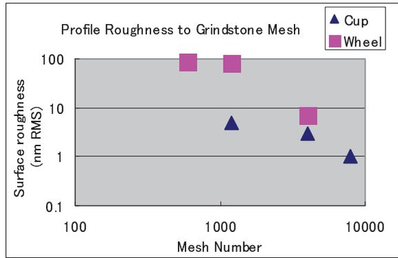
Fig.7: Roughness Derived from Line Profile.
