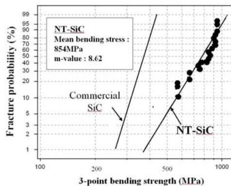
Fig.3 Weibull probability plot for 3-point bending tests
