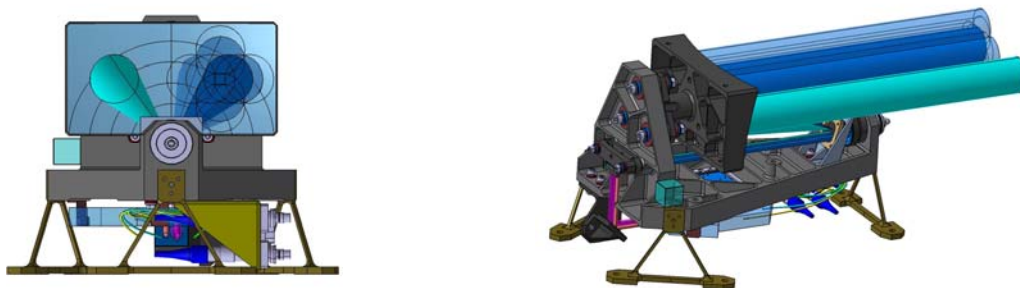
Fig. 3.: Optical head consisting of telescope on top and beam-combiner bench below central base plate. An intermediate field stop at the focus of the Dall-Kirkham is implemented allowing operation close to sun direction. The receive aperture is tolerant to lateral beam shifts.
