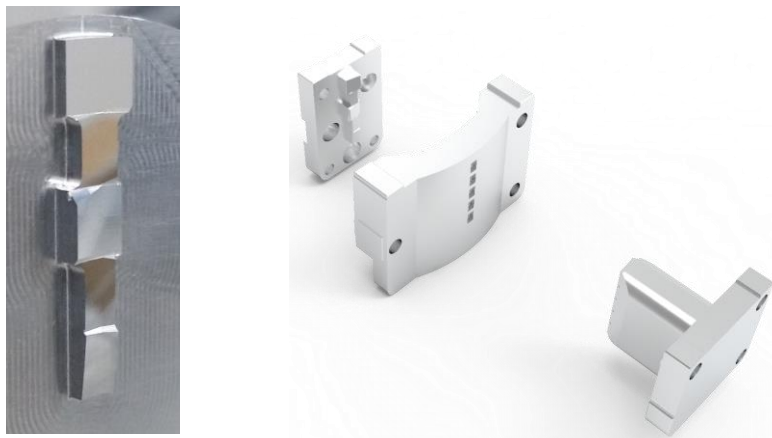
Figure 10 (left) prototype SPEXone telescope M2t, (right) rendering of telescope showing from left to right M2t, M1t, M3t.
