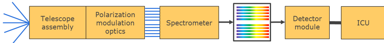
Figure 2 SPEXone multi-angle polarimeter instrument building blocks along the signal path; five-viewing angle telescope assembly, polarization modulation optics module, spectrometer module projecting two orthogonally polarized spectra per viewing direction, detector module that records the ten spectra and instrument control unit.
