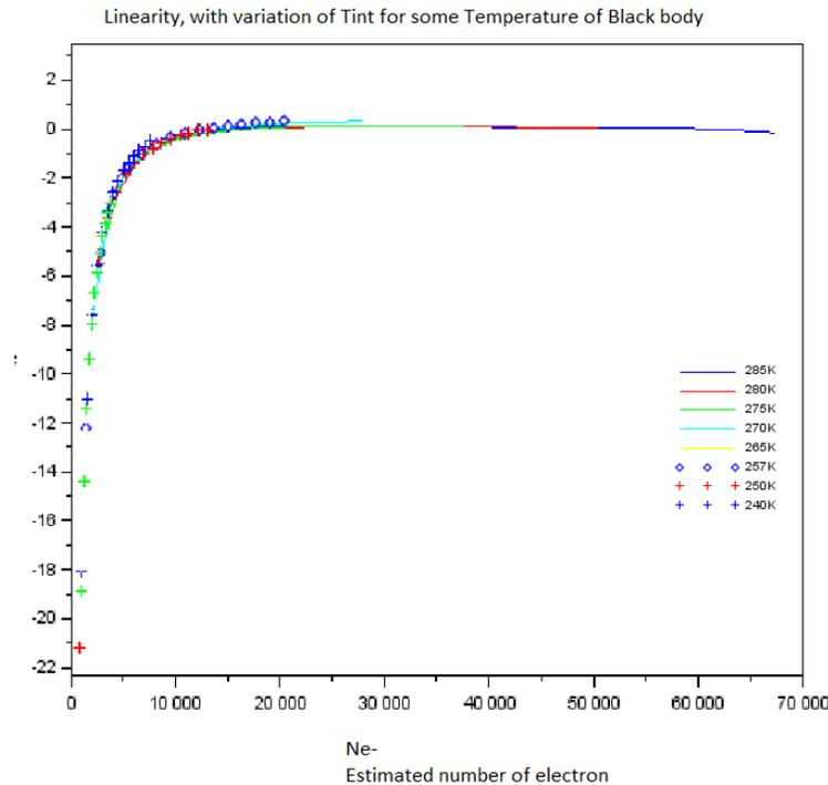
Figure 11 : NL at matrix level (Integration time variation)
