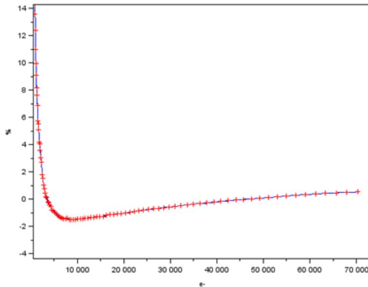
Figure 8 : matrix level non linearity (illumination variation)
