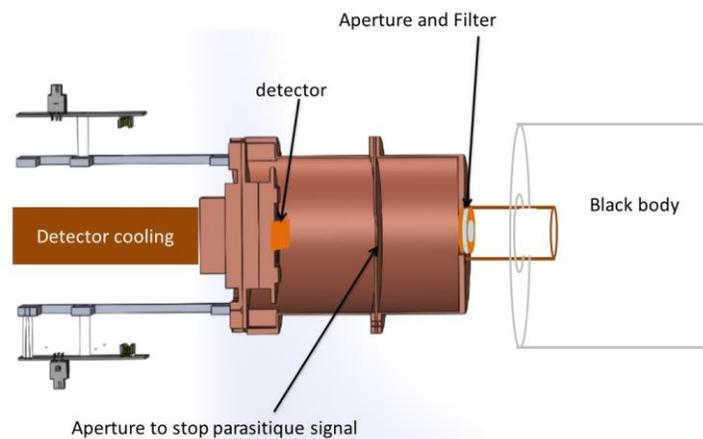
Figure 5: detector Housing
