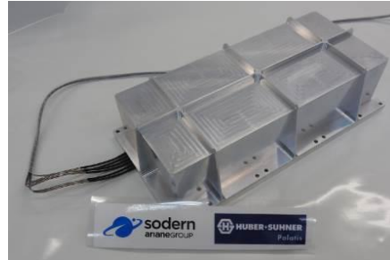
Figure 4-3 Picture of the OPTIMA 48-port switch breadboard
