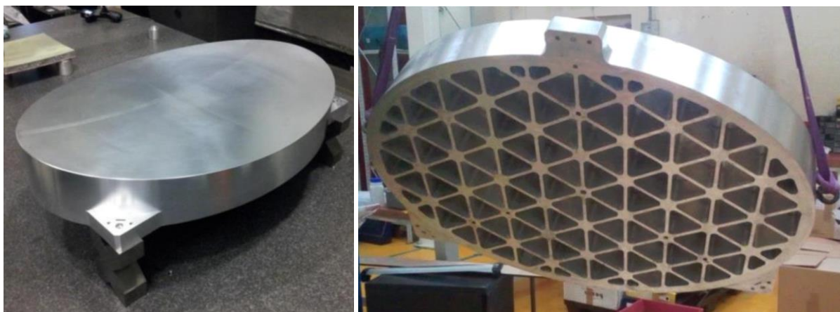
Figure 3. Front (left) and backside (right) of the PTM mirror prototype after milling.
