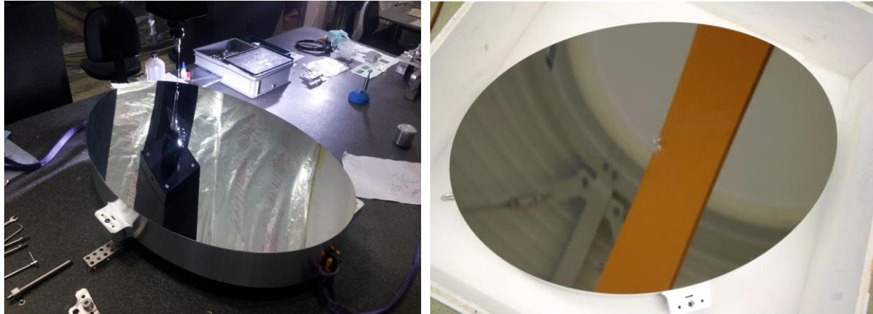
Figure 4. Two views of the PTM mirror surface after diamond turning.
