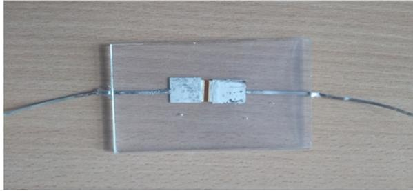
Figure 2. Photo of investigated PCSS switches made of semi-insulating gallium phosphide.
