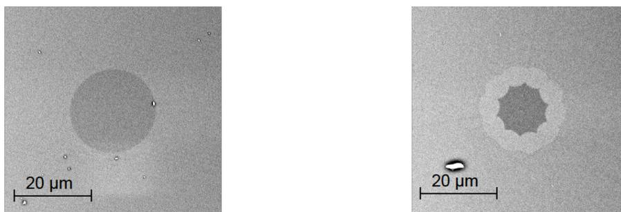
(a) SEM image of CREOL made 25/400  $\mu\text{m}$  gain fiber (b) SEM image of the 25/400  $\mu\text{m}$  CDF under test
