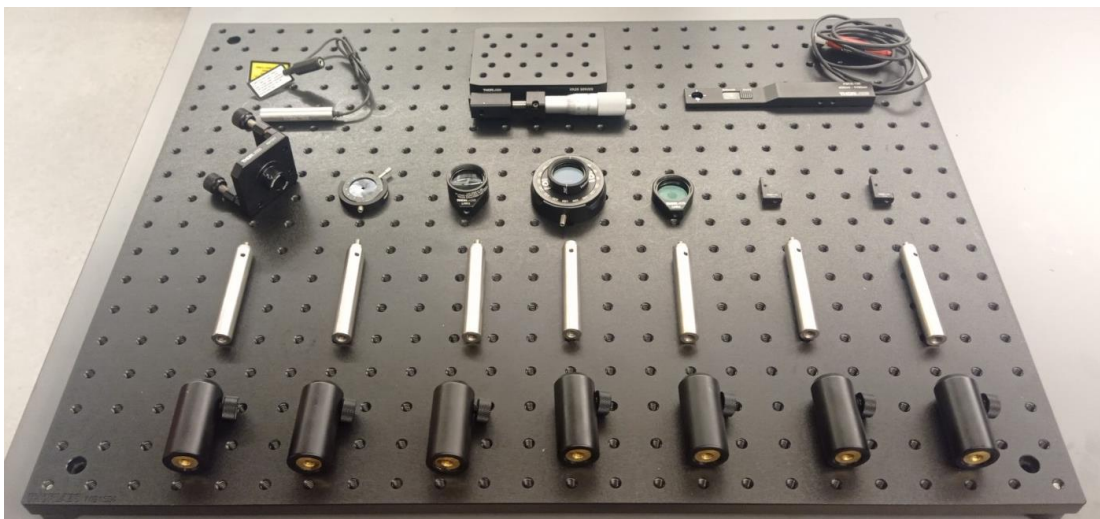
Figure 4. Laser, power meter, optical and mechanical components used in the fiber optics experiments.
