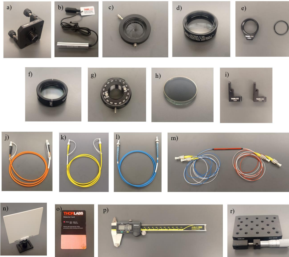
Figure 3. Parts are used in the fiber optics experiments. a) Laser Mount (KM100T), b) Laser diode (CPS635), c) Iris (ID20), d) Convex Lens (LA1608-A-ML), e) Lens Mount (LMR1), f) Half Wave Plate (WPH10ME-633), g) Rotational Mount (RSP1D), h) Polarizer (LPVISE100-A), i) Ferrule (FCM), j) Multi-mode fiber (M42L01), k) Single mode fiber (P1-460B-FC-1), l) polarization Maintaining fiber (P1-488PM-FC-1), m) Fiber Coupler (TW630R5F2), n) Viewing Screen (EDU-VS1), o) Viewing Card (VRC2), p) Caliper, r) Translational Stage (XR25P).
