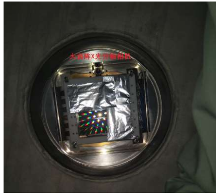
Figure 8. Performance calibration experiment photo of \Phi 106 X-ray framing camera
