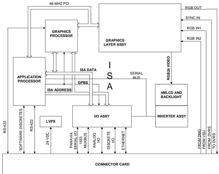
Figure 2.1-1 Multi-Processor Functional Block Diagram
