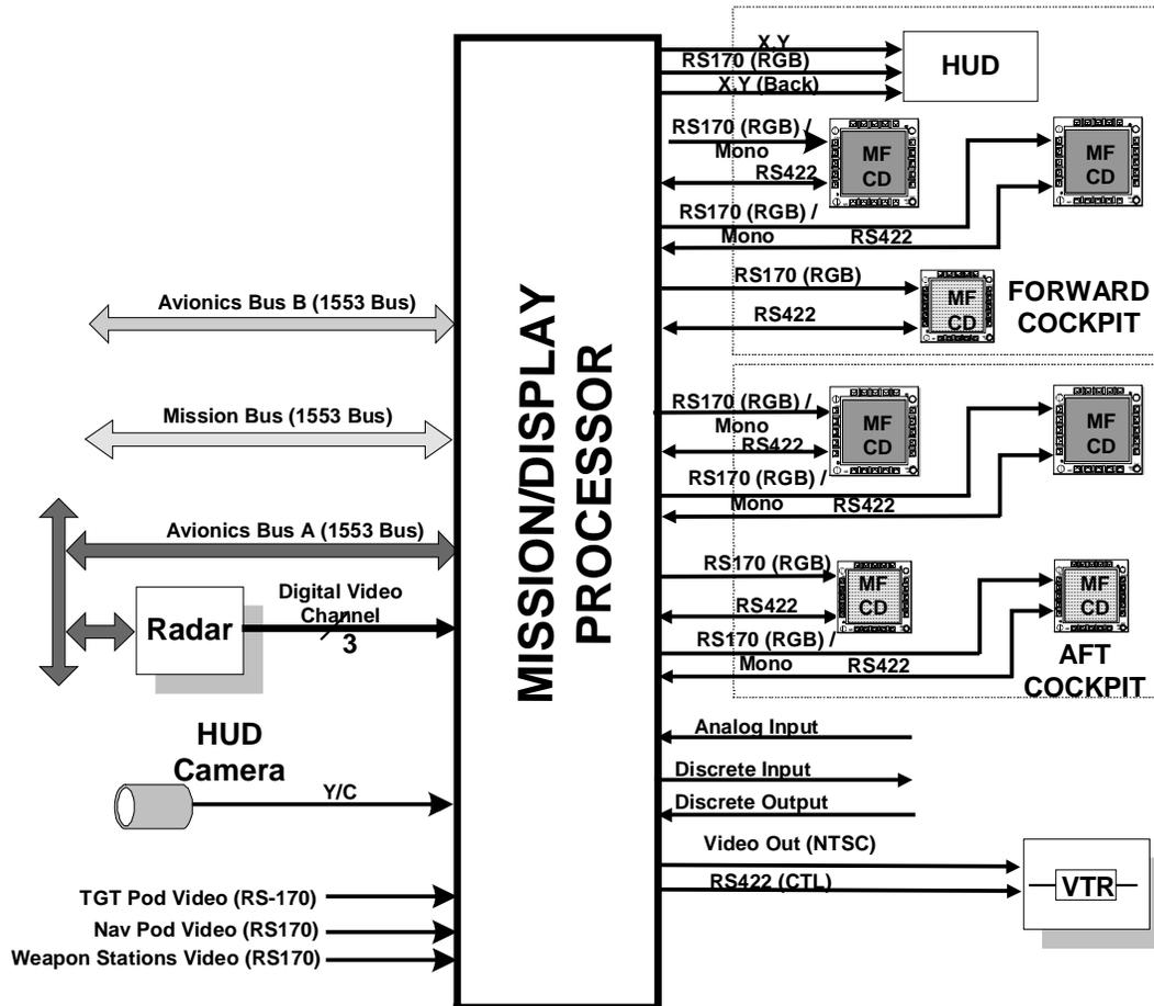
Figure 1.2-1 Hybrid System Block Diagram
