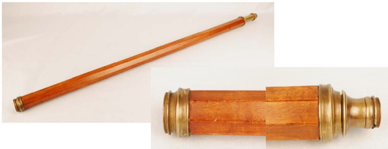
Figure 4. Reverse taper telescope (unsigned, circa 1750, English). The length of the telescope is 1090 mm; the barrel diameter is 33 mm on the objective end and 42 mm on the eyepiece end.
