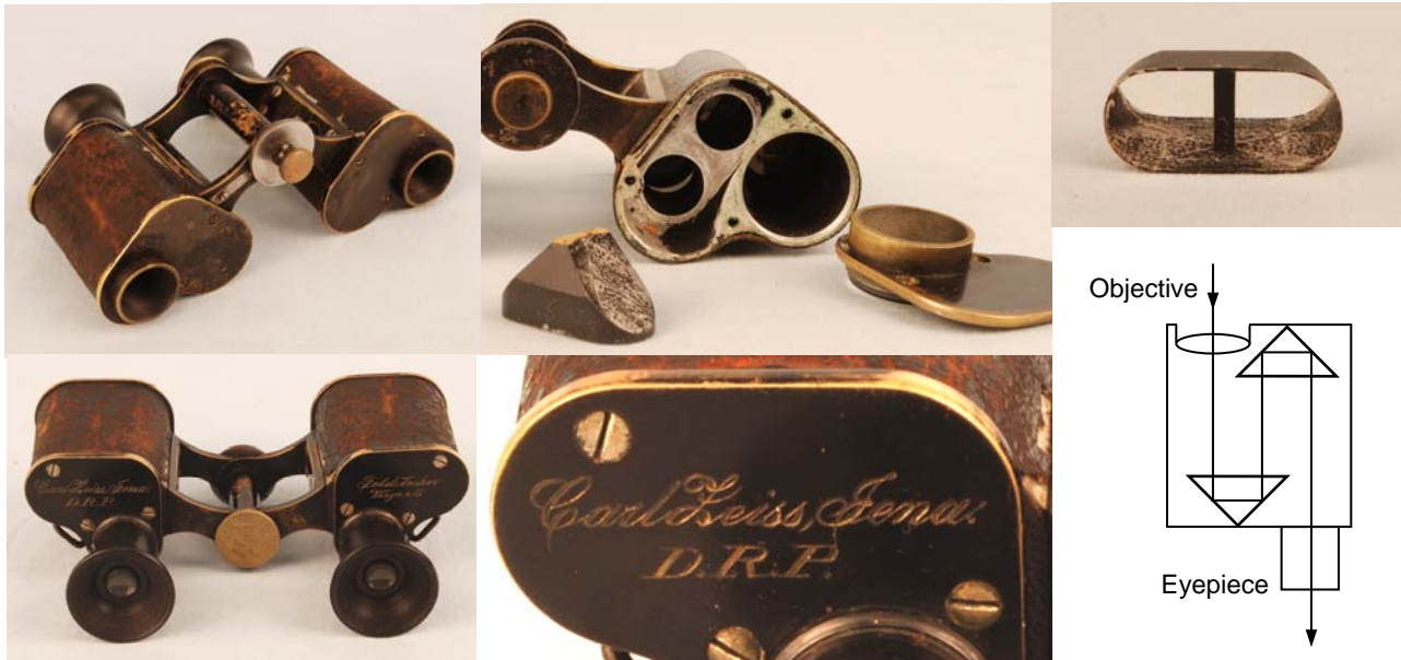
Figure 17. Zeiss 6X15 binoculars with serial number 306 (1895). The script inscription reads "Carl Zeiss, Jena D.R.P." and "Feldstecher Vergr = 6". The now-familiar Zeiss lens logo was first used in 1904. Removing the prism cover and the objective lens shows the prism mount and a Porro prism for a pair of 8X20 binoculars of the same era (No. 4976; 1897). The diagram shows the arrangement of the prisms in the housing. Of course, both prisms are actually rotated by 45 deg out of the plane. In this 8X pair, the prism separation is approximately 30 mm; the separation is approximately 20 mm in the 6X binoculars as the prism body is shorter.
