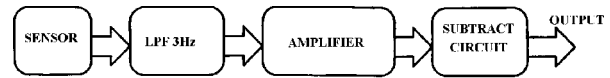
Fig. 2 Block diagram of the cardiac-rhythm detector. The sensor transduces the heart beat into an electrical signal. This is passed through a low-pass filter and then to an amplifier. The last stage is a rester circuit from which the output represents the cardiac rhythm.
