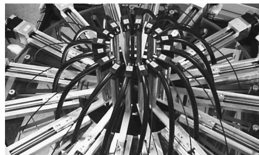
Fig. 2 The fiber-optic patient interface is shown. The larger black cables are the detector fiber-optic bundles. The fiber optics are mounted on posts connected to a series of translation stages mounted radially.
