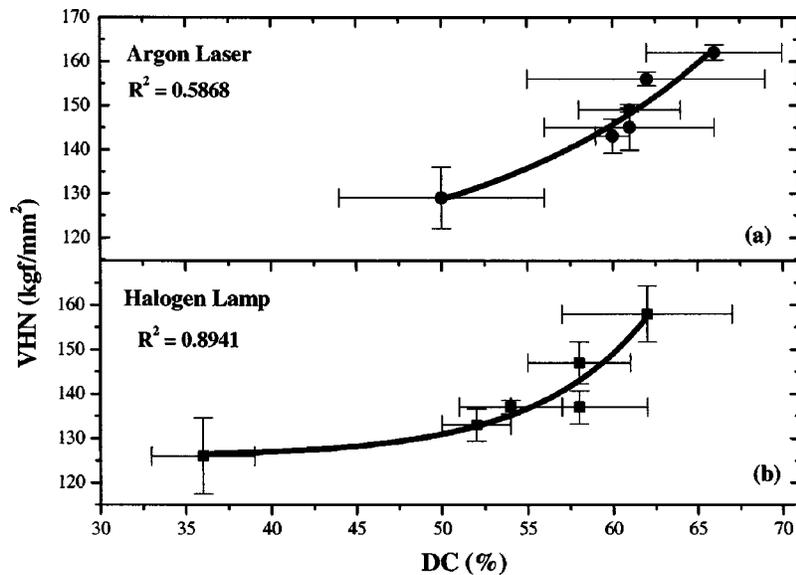
**Fig. 4** Correlation between the Vickers hardness number and the degree of conversion for irradiation using (a) an argon laser and (b) a halogen lamp.
