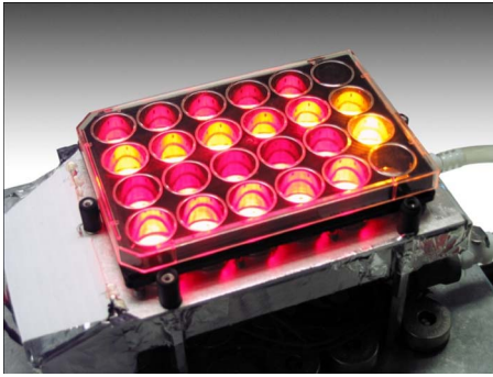
Fig. 1 Illumination device during photoactivation of fibroblasts cells in the 24-wells plate.
