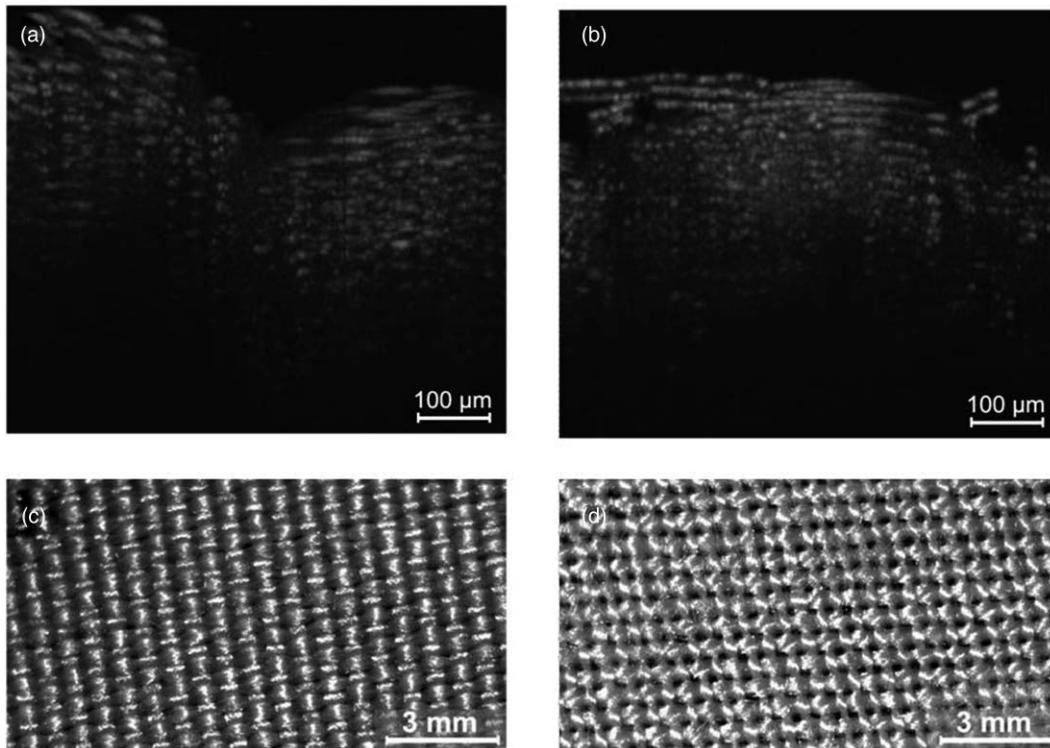
**Fig. 1** (a) Characterization by optical coherence tomography OCT picture of polyamide fabric. (b) Characterization by optical coherence tomography OCT picture of polyester fabric. (c) Top view picture captured by Primos system of polyamide fabric. (d) Top view picture captured by Primos system of polyester fabric.
