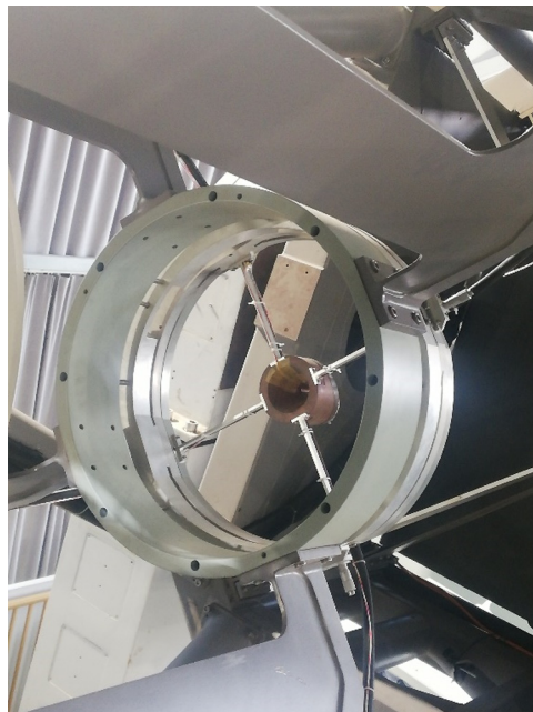
Fig. 4 Structure of the heat-stop for CLST.
