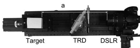
**Fig. 2** Simple optical setup to demonstrate the feasibility of the novel TRD-3D-SIM. In the figure, “*a*” indicates the working distance (WD).
