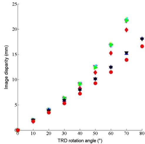
**Fig. 4** Image disparity as a function of TRD angle at WD of 153 and 250 mm. In the figure, yellow upward triangle: “L” angle and 250 mm WD, pink downward triangle: “R” angle and 250 mm WD, green left triangle: “R” angle and 153 mm WD, turquoise left triangle: “L” angle and 153 mm WD, red diamond: theoretical data, blue upward triangle: “E” angle and 153 mm WD, black downward triangle: “E” angle and 250 mm WD, and red circle: theoretical data.
