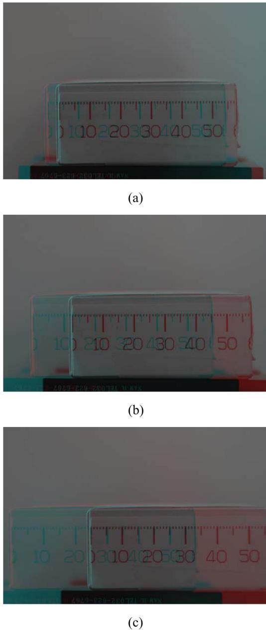
**Fig. 3** 3-D stereoscopic images of a target at the TRD angles of (a) E 20 deg, (b) E 60 deg, and (c) E 100 deg. “E” indicates the angle equally rotated both clockwise and counter-clockwise. For example, E 10 deg means rotated  $-5$  deg (clockwise) for the right image and rotated  $+5$  deg (counter-clockwise) for the left image.
