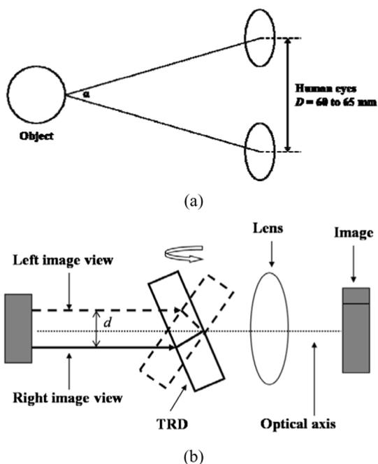
**Fig. 1** (a) Schematic diagram of an adequate stereoscopic viewing condition for a human. (b) Schematic diagram of the transparent rotating deflector (TRD) action in three-dimensional (3-D) stereoscopic imaging modality (SIM) in which solid and dotted lines indicate the viewing angles of right and left images, and “*d*” indicates the image disparity between the right and left images, which can be varied by adjusting the rotation angle of the TRD.
