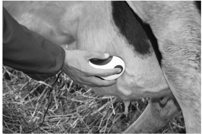
Fig. 1 Measurement of dermal carotenoid concentrations on the bovine udder skin using a portable LED skin scanner system.
