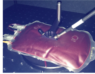
Fig. 2 Diffuse reflectance measurement of ES unit inside the dark box. The reflection probe was placed in the 45-deg aperture of the probe holder. The probe holder was tightened at the point where the probe connects the surface of the blood bag.
