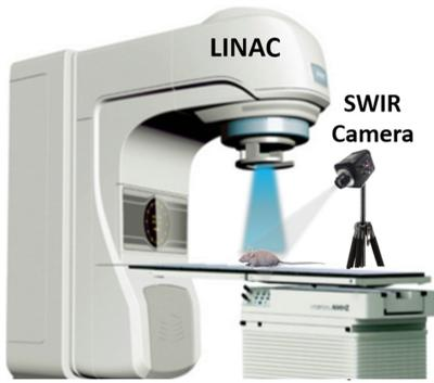
Fig. 1 Imaging setup for CESFI with an electron beam (blue).
