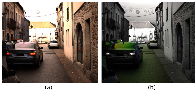
Fig. 9 (a) White-balanced color image. (b) Fake colors image representation for the red channel.
