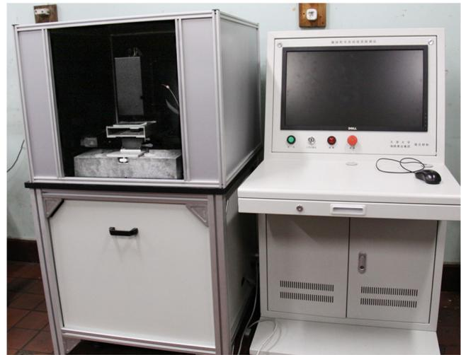
**Fig. 1** Video-based inspecting instrument for watch escapement (VIIWE).
