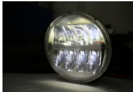
Fig. 18 A headlamp containing upward pcW-LEDs for the high beam and downward pcW-LEDs for the low beam.
