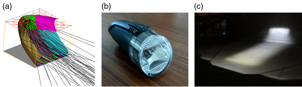
Fig. 17 (a) The structure of the reflector, (b) a photo of the bicycle headlamp, and (c) the projected light pattern. 88
